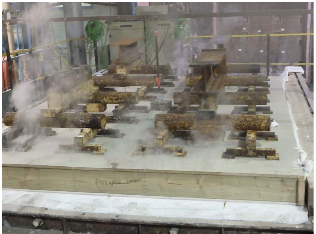
The unexposed surface of the assembly after a test duration of 30 minutes
