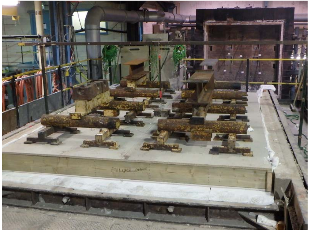
The unexposed surface of the assembly after a test duration of 15 minutes
